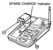
The spare battery is always being charged in the base unit while the AC adaptor is connected. The battery cannot be overcharged.
