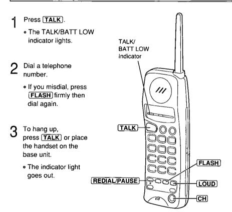
If an alarm tone sounds in step 1, move toward the base unit or place the handset on the base unit. Then try again.
